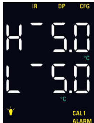
Dew point alarm configuration
