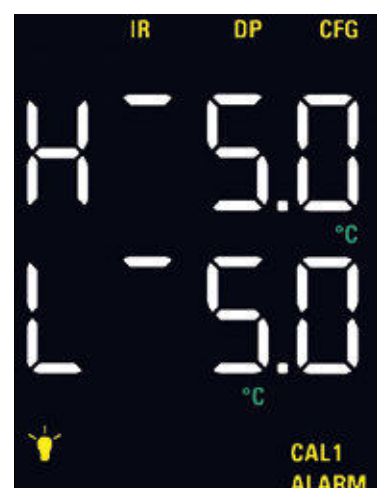
Dew point alarm configuration
