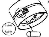
Note: The standard CEI R6 or LR6 battery lasts for more than a year at 23°C. Use a waterproof alkaline type battery.
